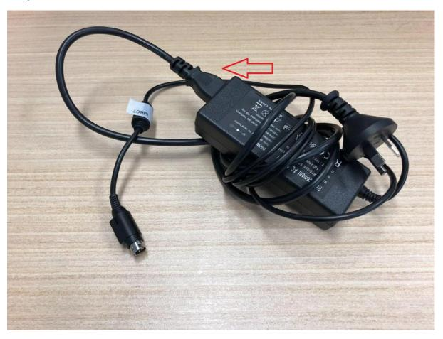
Take the power cable out from the AC adapter and leave it for 5 minutes.
