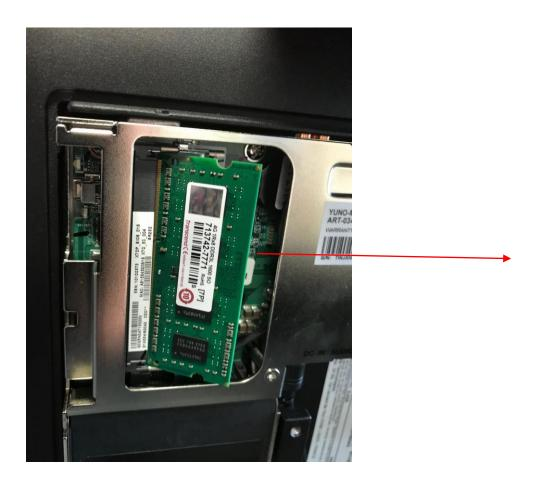
Important: Handle the new memory by the side edges only, avoiding the gold connector strip. Place new memory in slot (make sure that you can't see the gold strip any more) and push lightly on top and bottom until the clips click into place.
